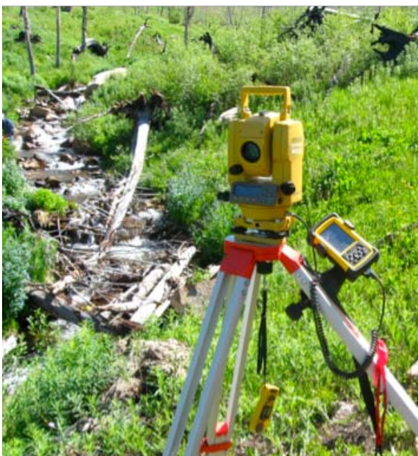
Figure 2. View of total station and channel filled with woody debris.
